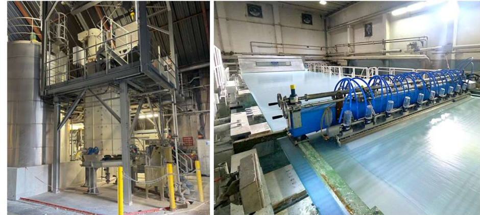
Image: 3-meter-wide surface applicator operating on a paper machine running at 500 m/min
