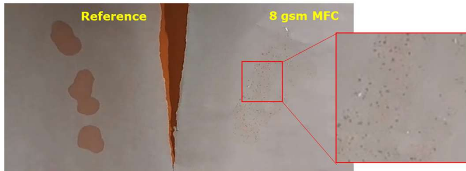
8 gsm MFC (Day 1) – Droplet test with Oleic Acid during trial.
