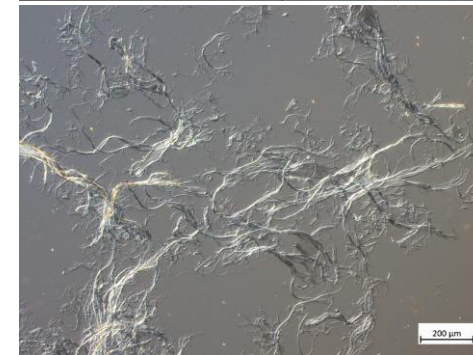
Optical micrograph showing MFC coarse macrostructure
