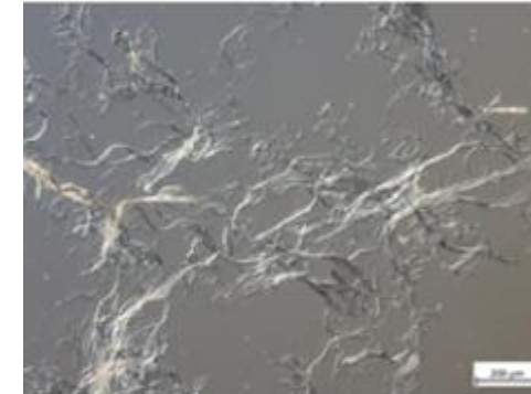
Optical micrograph showing MFC coarse macrostructure
