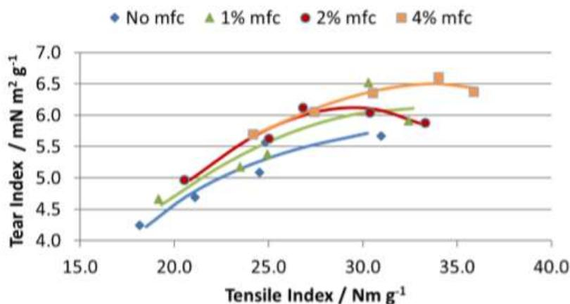
**6. Impact of MFC dose on Tensile and Tear strength at 20% filler and increasing refining.**
