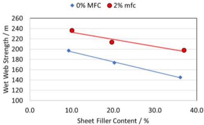
5. The effect of MFC addition on initial wet web strength from pilot machine trial.
