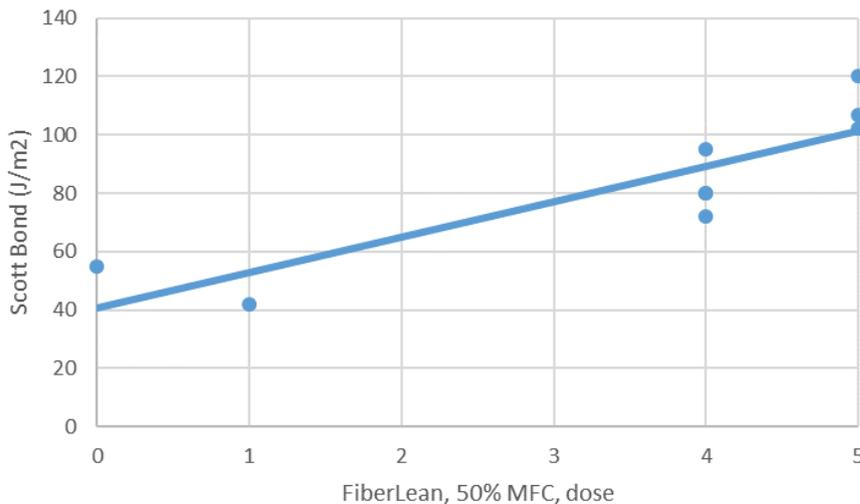
**Figure 3, Folding Boxboard mechanical pulp middle layer Scott Bond vs % FiberLean dosage, full scale results.**
