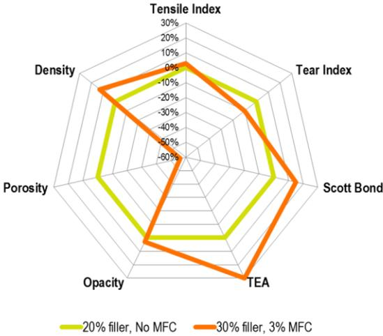
**Figure 2. The base effect of using MFC-mineral composite to increase filler loading 10% units in UWF.**
