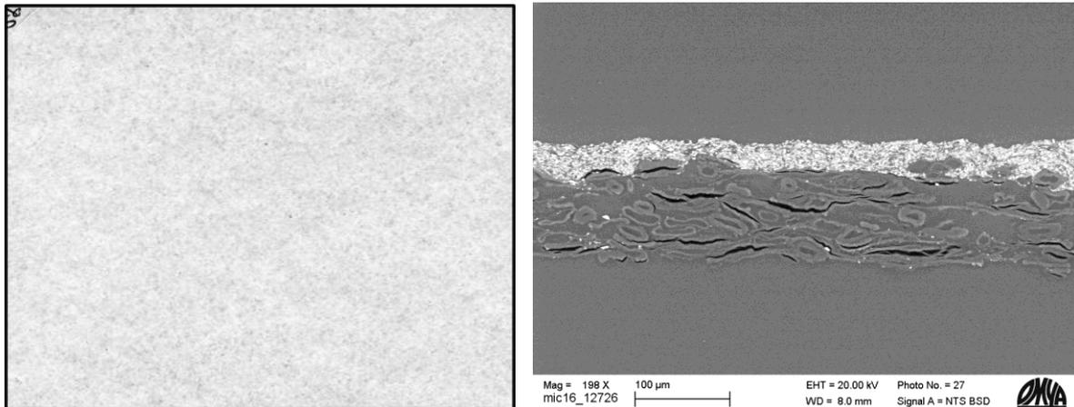
**Figure 4 a, Surface picture of wet-end coated kraftliner with brightness exceeding current Coated White Top Kraftliner specifications at ca.40 g/m<sup>2</sup> coat weight. b, Cross section view of wet-end coated kraftliner showing minimum coating penetration despite the open base structure.**
