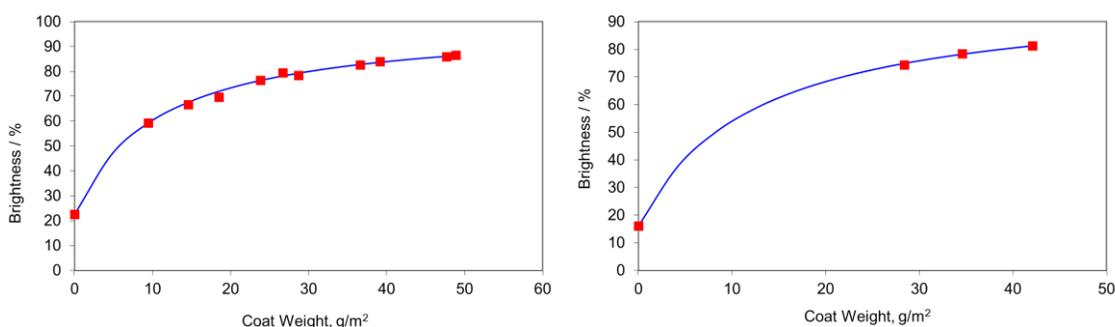
**Figure 4. Brightness vs coatweight for 80%  $\text{CaCO}_3$ /20% mfc on unbleached Kraft base, fitted to Kubelka-Munk model. Handsheet data (left), Pilot machine data (right)**
