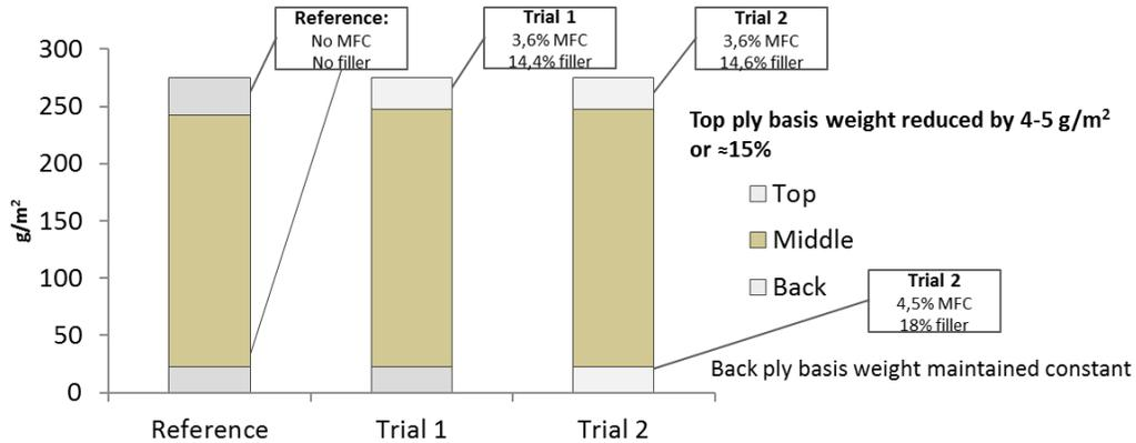
**Figure 2. Mill trial results using co-ground mineral and mfc to increase filler loading in the outer layers of folding box board**
