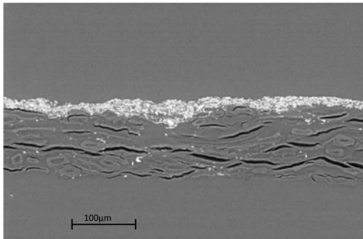
**Figure 3. SEM Cross section of unbleached long fibre Kraft linerboard with 28gsm coating of 80% CaCO<sub>3</sub>/20% mfc applied at the wet end**
